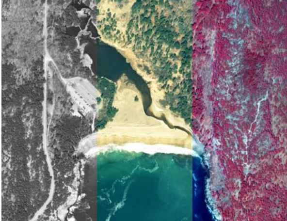
Black & white, true color, and Color Infrared imagery simultaneously captured with a digital camera for the Town of Bar Harbor, ME in April 2008. Sand Beach, Acadia National Park, ME. Courtesy of Kappa Mapping, Inc.
